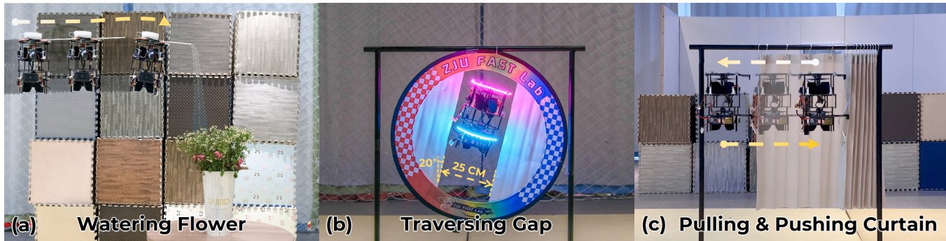
Fig. 1: Our proposed FLOAT Drone demonstrates diverse close-proximity operation tasks. (a) Carrying a watering can and watering flowers via a tilted hovering posture. (b) Traversing a narrow gap inclined at 20 degrees, with a width of 25 cm. (c) Pulling and pushing a deformable curtain within a minimum workspace of only 30 cm.
